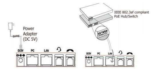
Note: If POE is available, the phone doesn't need to connect to the AC power adapter.
