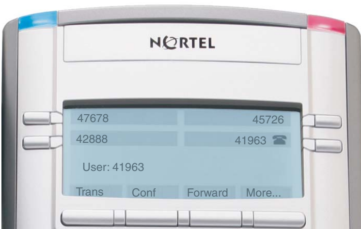
Figure 9: Logged in to an IP Phone 1150E using an IP Phone 1120E
