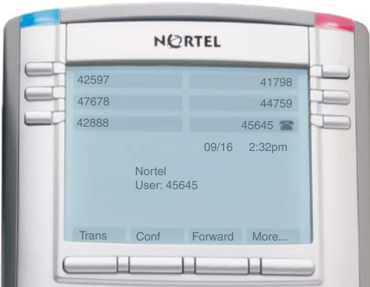
Figure 8: Logged in to an IP Phone 1150E
