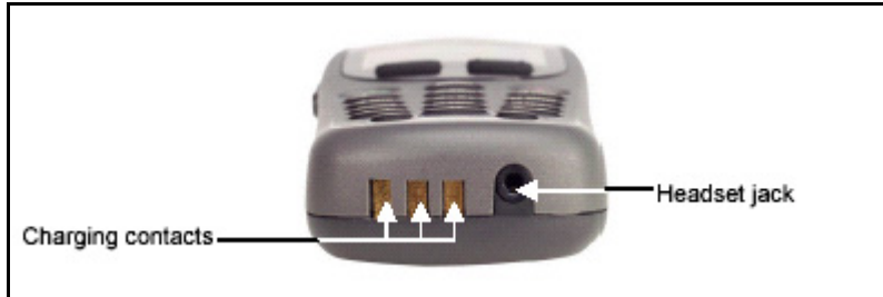
Figure 2 WLAN Handset 2210 bottom view
